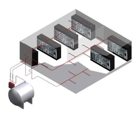
The typical arrangement of this equipment is as follows: low-pressure tank, pipework and application nozzles.
